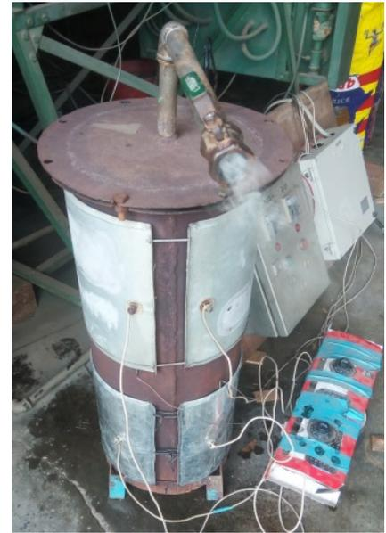
**Figure 1.** The torrefaction reactor.
