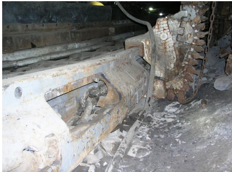
Figure 2. Subject of measurements: coal plough system at LW Bogdanka.
