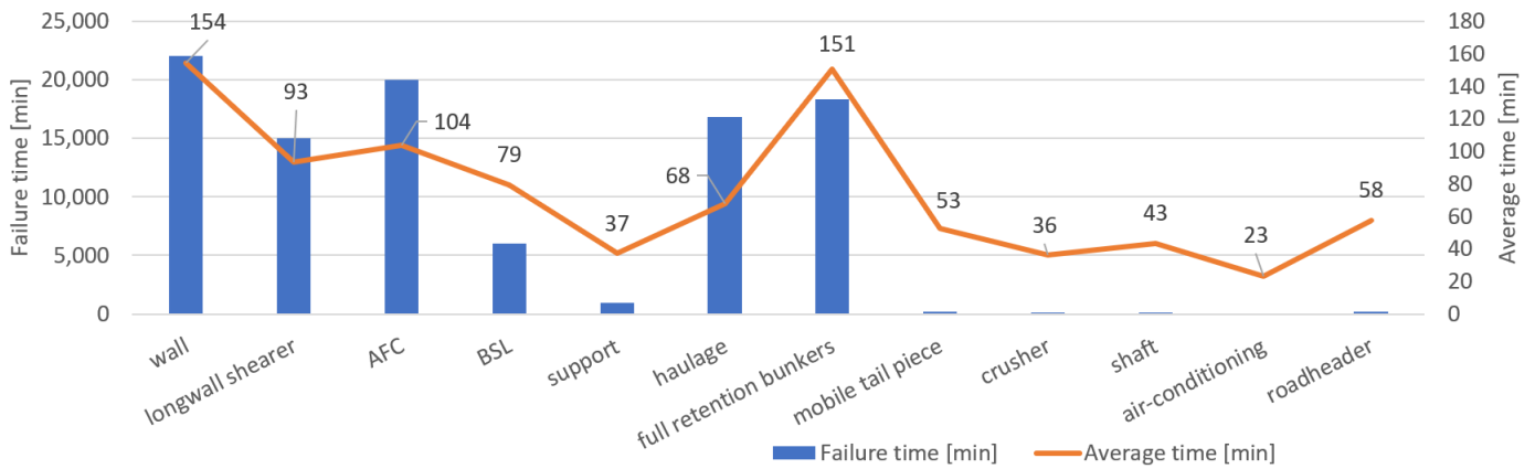
Figure 5. Duration of failures and average duration of failures of shearer longwalls in total.
