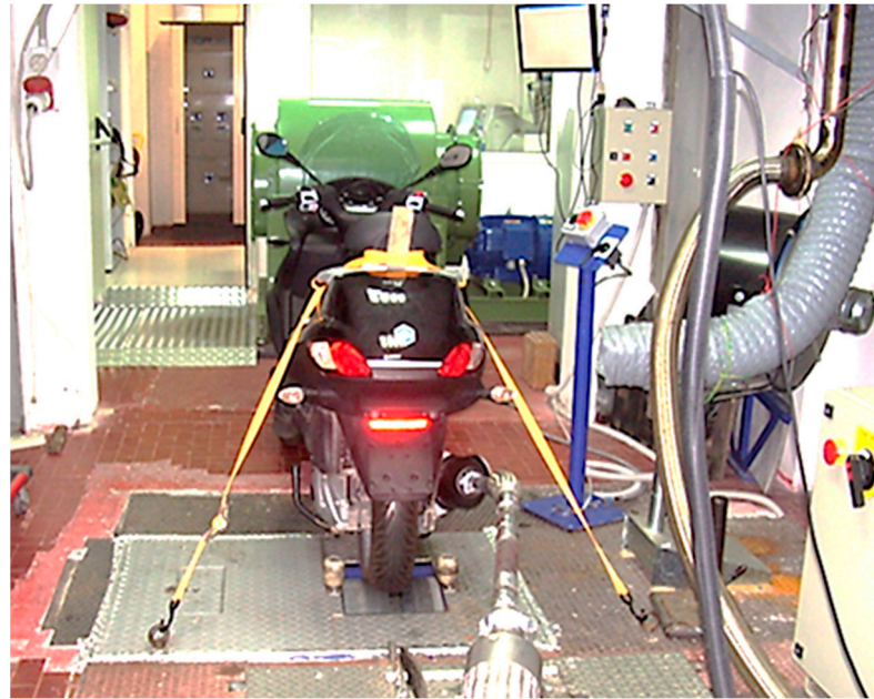
Figure 1. The motorcycle under examination on the test bench.
