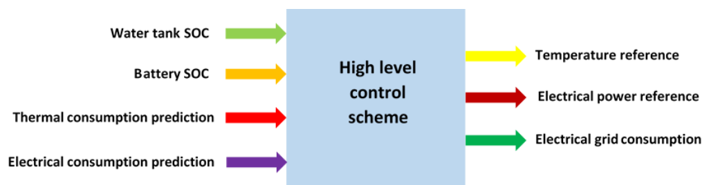
Figure 6. Control scheme for the CHP system.
