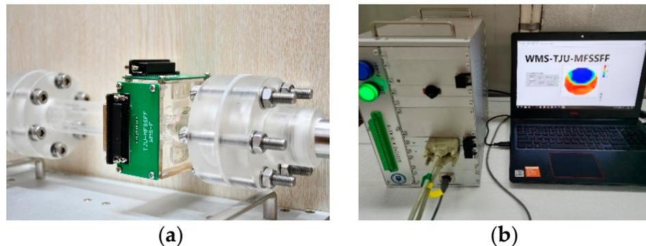
**Figure 3.** Wire-mesh sensor system used in this study: (a) Wire-mesh sensor; (b) Sensor system.
