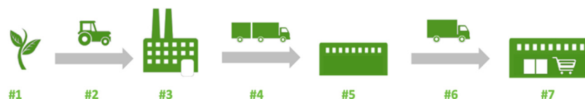
Figure 1. Sample supply chain. #1: raw material supplier, #2: single-drop transport from the supplier to the producer, #3: producer (with raw material and finished product warehouses), #4: single-drop transport from the producer to the distribution center, #5: distribution center, #6: multidrop transport from the distribution center to the retailer, #7: retailer (with a backroom warehouse and a display area).
