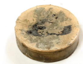
Figure 5. Disc-shaped samples were used to check thermal conductivity (photo by K. Seńczuk).
