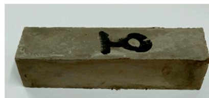
Figure 7. Beam used in flexural strength test (photo by K. Seńczuk).
