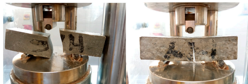
Figure 8. Samples used in compressive strength tests (photo by K. Seńczuk).
