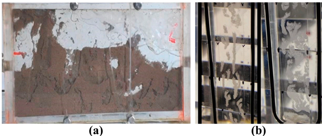
Figure 17. The accumulation pattern of proppant particles in rough fractures (a) different layers of sand-packing profile [41], (b) buildup of cellulose fibers in the hydraulic fracture [42].
