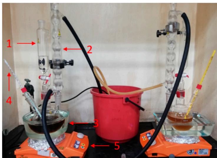
Figure 2. Experimental system reported in [11], including (1) a methanol/KOH mixture container, (2) reflux condenser, (3) heating bath, (4) temperature controller, and (5) magnetic stirrer.
