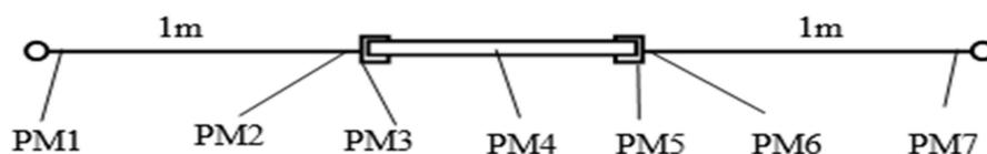
**Figure 6.** Arrangement of measuring points.
