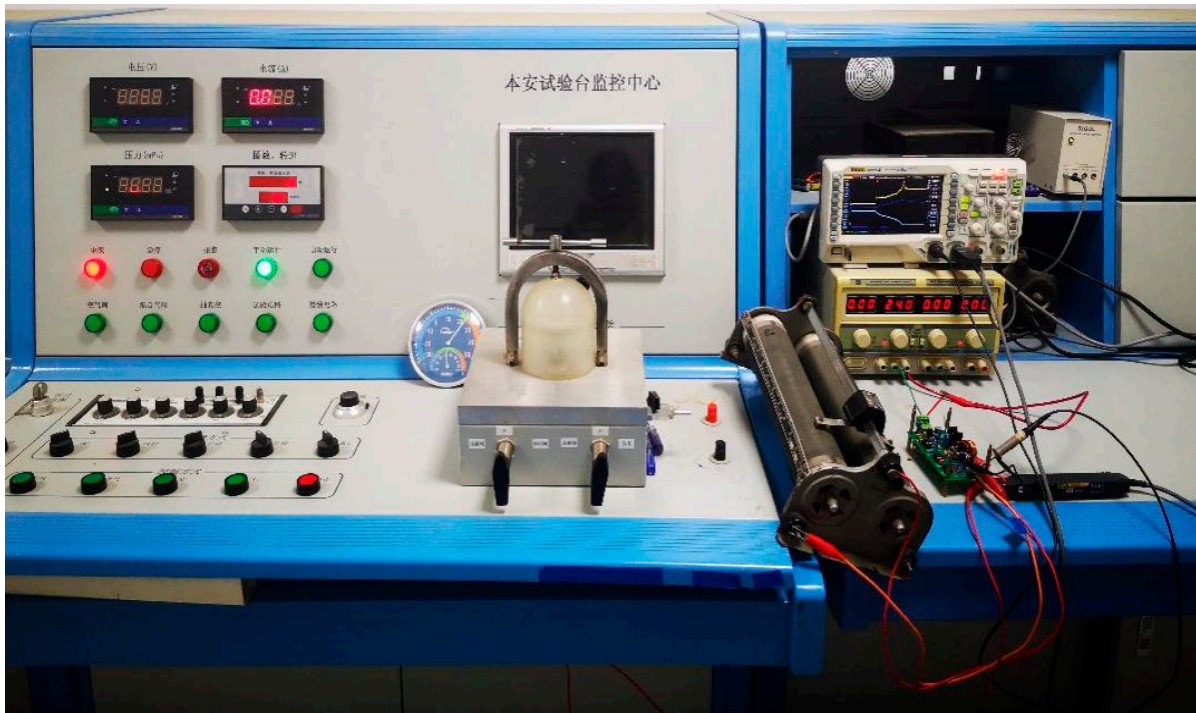
Figure 8. Intrinsically safe spark test device.
