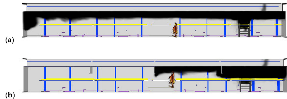
Figure 10. Smoke in a 180 m long turbine house and a height of 30 m. (a) No smoke curtains, (b) 8-m high curtains from the roof.
