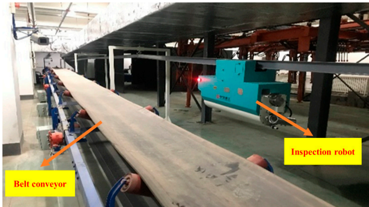
Figure 8. Working diagram of the underground inspection robot in coal mine.
