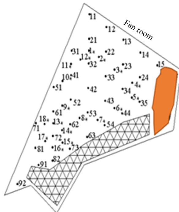
Figure 10. Distribution map of borehole detection points in coal gangue hill.
