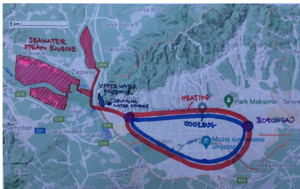
Figure 3. Layout of the collector fields of SSE technology (which uses Sava River as input water) and distribution loops of heating and cooling for the city of Zagreb.
