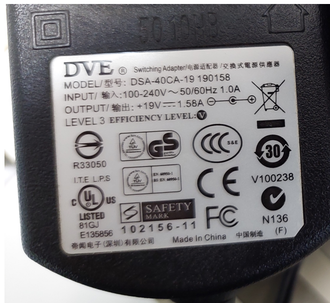
Figure S2: Power supply DVE DSA-40CA-19
