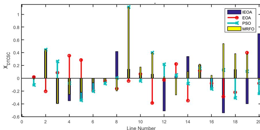
**Figure 6.** Optimal size of DTCSC using different algorithms in solving scenario one for 14-bus system.
