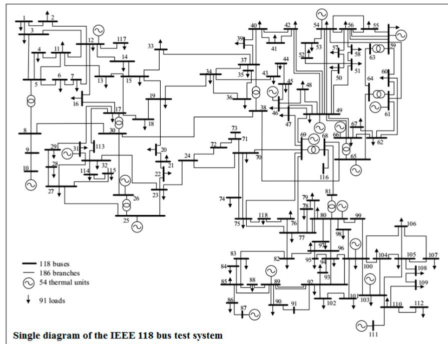
Figure 11. Schematic of IEEE 118-bus system.
