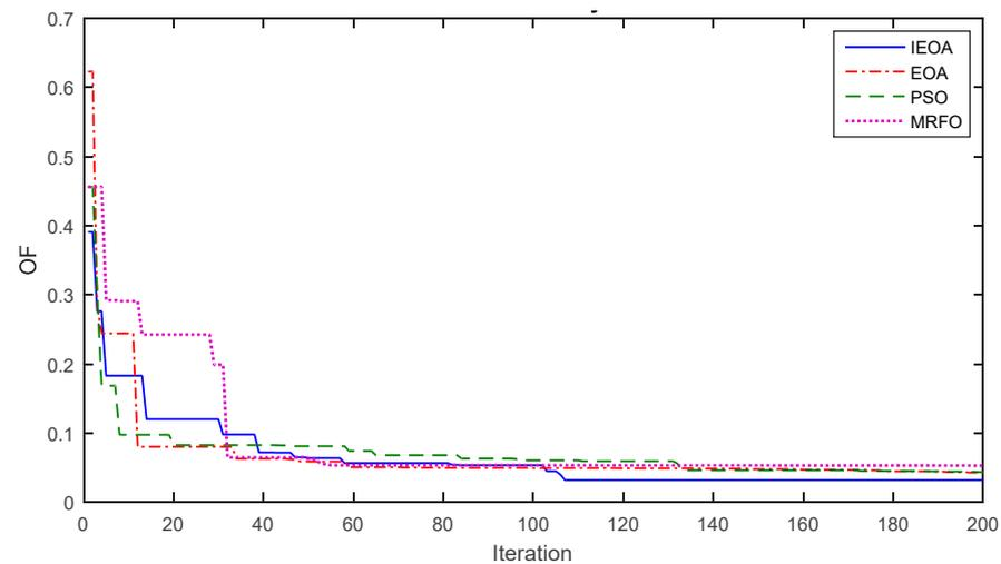
**Figure 5.** Convergence curve of different algorithms in solving scenario one for 14-bus system.
