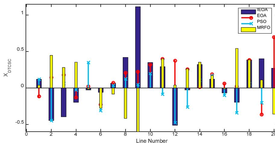
Figure 8. Optimal size of DTCSC using different algorithms in solving scenario two for 14-bus system.
