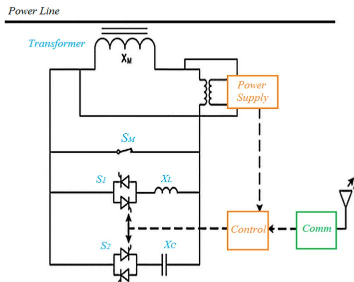
**Figure 2.** Circuit scheme of the DTCSC.
