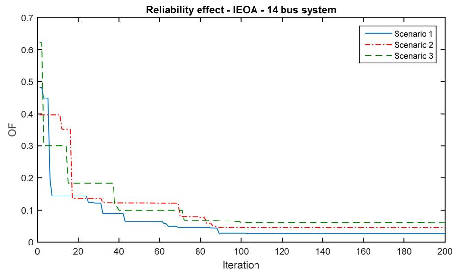
**Figure 13.** Convergence curves of different algorithms for 14-bus system considering reliability.
