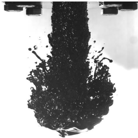
Figure 1. Woods metal jet breakup in water: T_j = 85\text{ }^\circ\text{C} , T_1 = 40\text{ }^\circ\text{C} , D_j = 50\text{ mm} , V_{j,in} = \sim 1.0\text{ m/s} [13].
