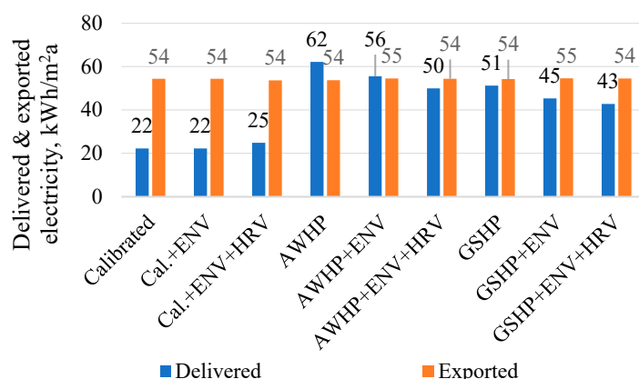
Figure 8. Yearly delivered and exported energy for a reference single-family house for different cases.
