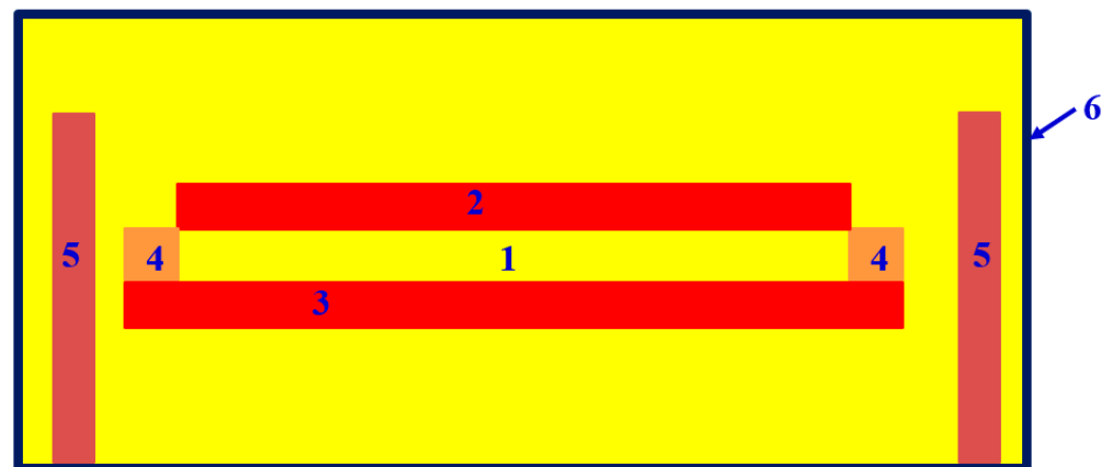
Figure 1. Diagram of the system for testing the insulating oil electrical properties. 1—mineral oil, 2—measuring electrode, 3—voltage electrode, 4—spacers (6 pieces), 5—moistened oil-impregnated pressboard placed in the vessel in the second series of tests and 6—hermetic vessel.
