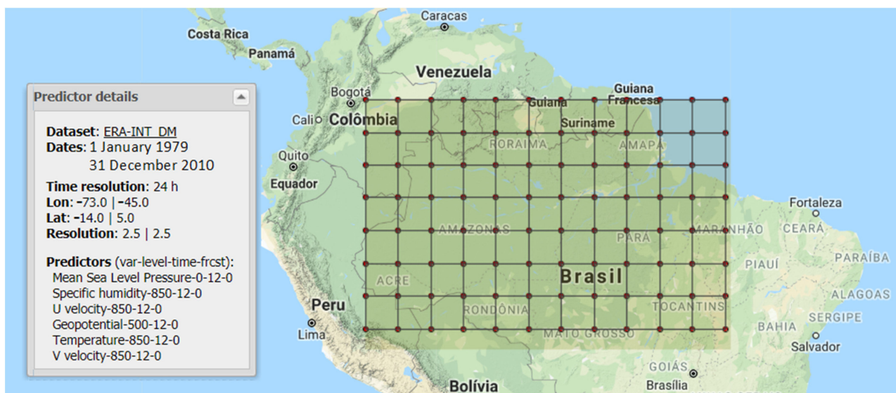
Figure 2. Resolution grid over the Amazonian area used to establish the relations between predictor (reanalysis) and predictand (surface observations) data.
