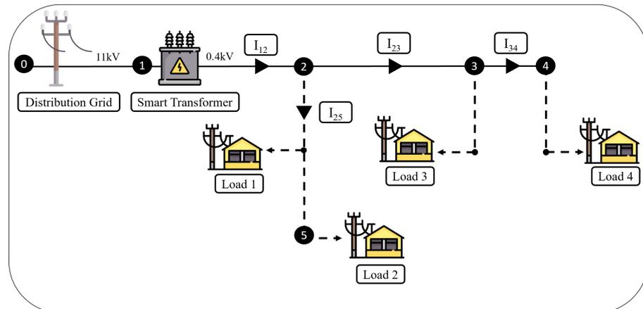
**Figure 1.** Feeder network system for one area.
