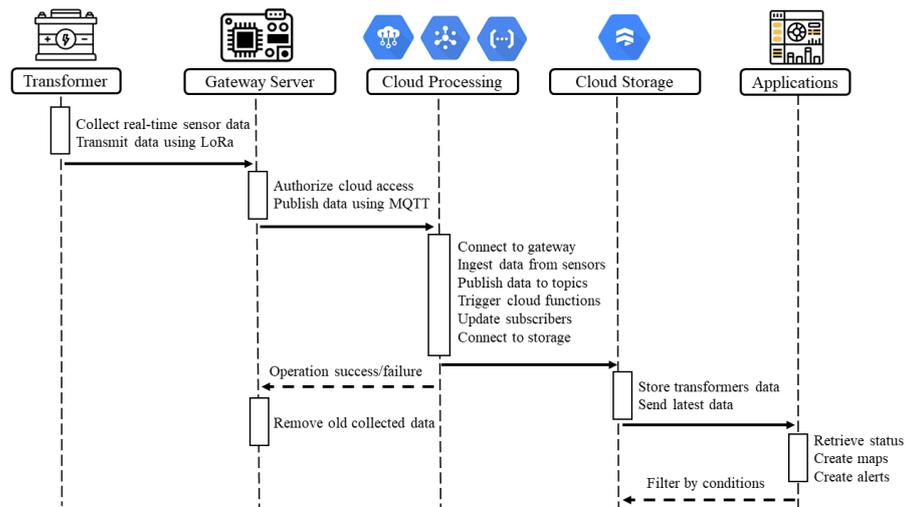
Figure 3. Sequence diagram of the system.
