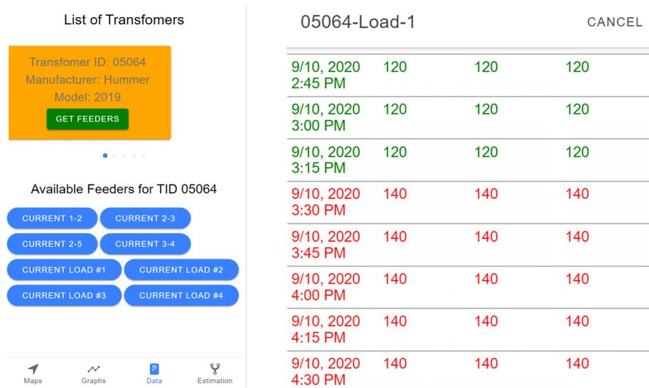
**Figure 5.** List of transformers and feeder current values on mobile application (green: normal, red: anomaly).
