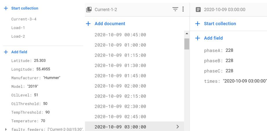
Figure 4. Transformer data available in cloud storage.
