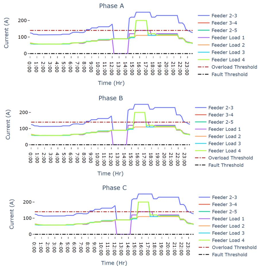
**Figure 6.** Graph visualizations of feeder current values on mobile application.
