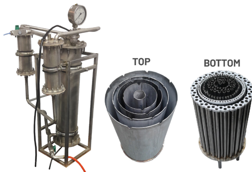
Figure 1. View of the investigated alkaline electrolyzer.
