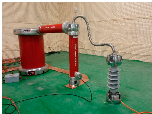
Figure 5. The experimental setup for the leakage-current measurement in a laboratory.
