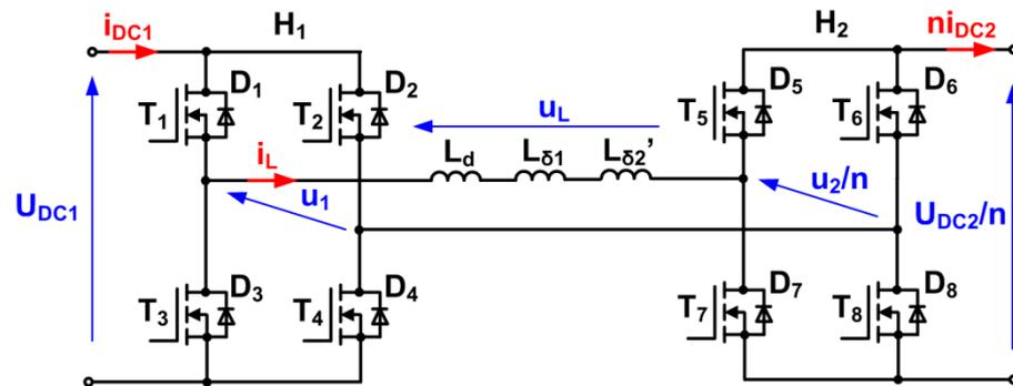
Figure 2. Equivalent circuit of the single-phase DAB converter.
