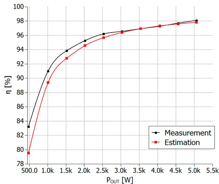
**Figure 14.** The estimated and measured energy efficiency characteristics of the tested DAB converter.
