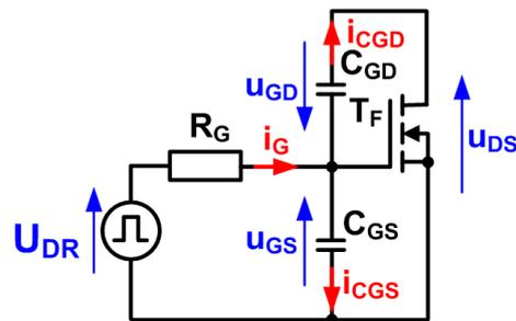
**Figure 8.** A gate circuit of the MOSFET transistor.
