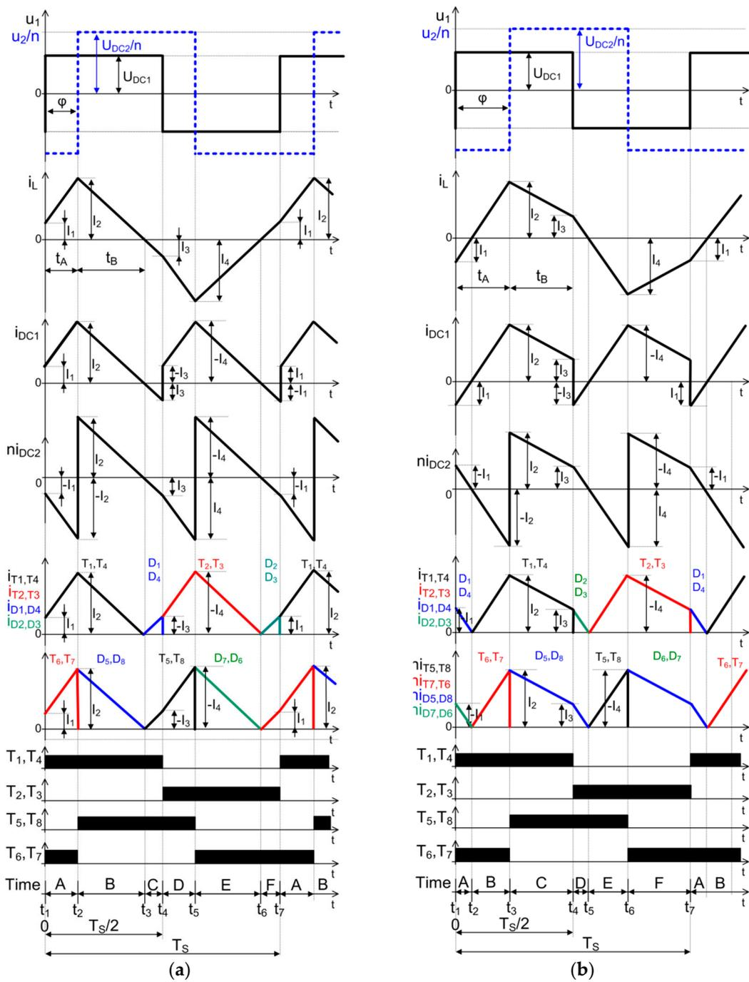
**Figure 4.** Simplified voltage and current waveforms of the DAB converter for  $U_{DC1} < U_{DC2}/n$ : (a) with  $I_1 > 0$ ; (b) with  $I_1 < 0$ .
