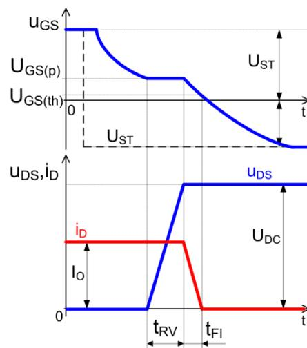
Figure 9. Voltage and current waveforms in a basic switching cell during the transistor turn-off process.
