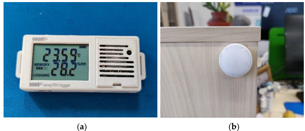
Figure 4. (a) HOBO temperature and humidity sensors, (b) Mijia light sensors.
