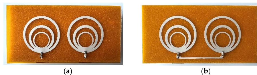
Figure 6. The 1 \times 2 RAA prototypes. (a) Without \pi -stub. (b) With \pi -stub.
