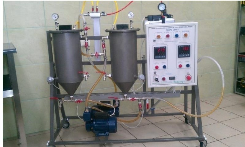
Figure 1. GW 201 reactor used to produce AFBE and AFME from leather waste.
