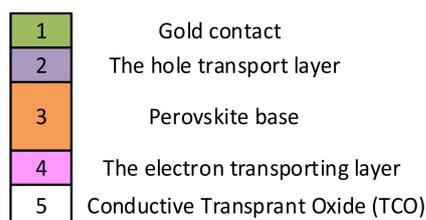
**Figure 10.** An example of a planar structure of a perovskite-based photovoltaic cell [1].
