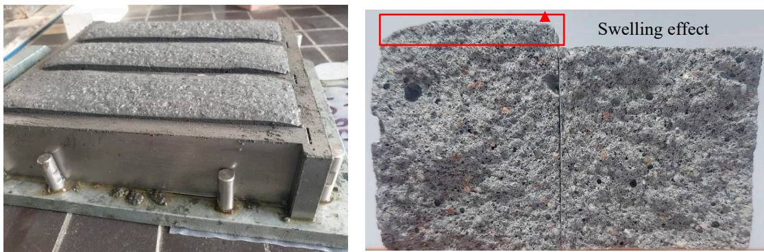
Figure 7. Swelling of the cement mortar with the addition of 18% fly ash.
