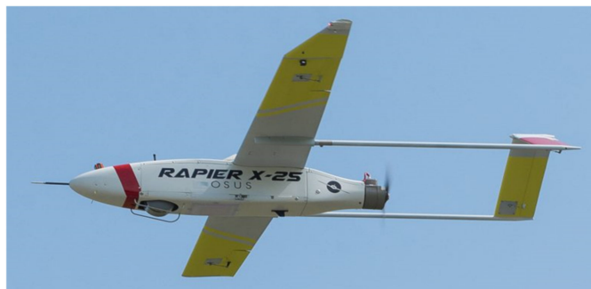
Figure 1. Lightweight fixed-wing UAV “Rapier X-25” by Sky Eye Systems (Cascina, Italy).
