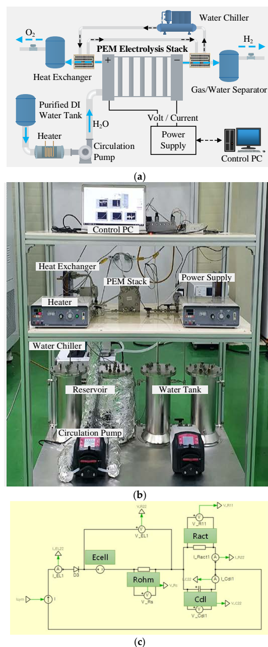
Figure 15. A 400 W class commercial PEMEL system configuration (a) simplified diagram, (b) actual configuration, and (c) electrical equivalent circuit modeling.
