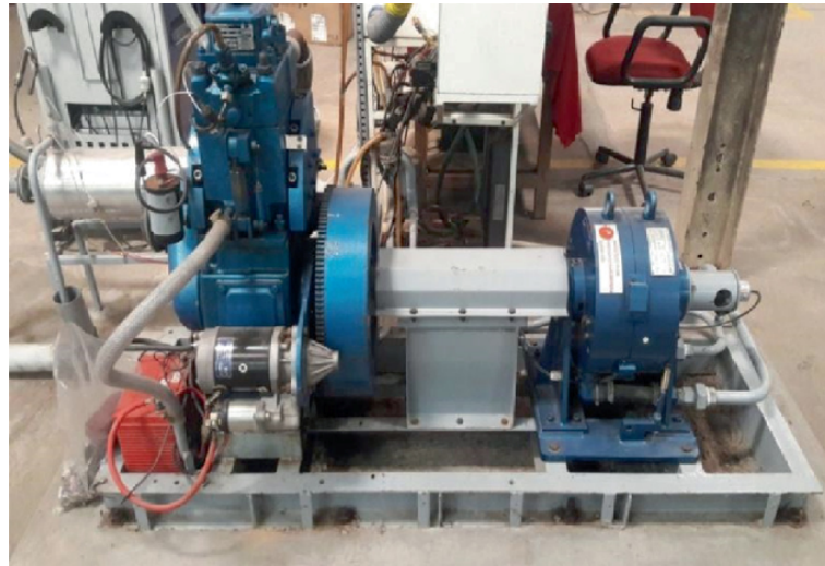
Figure 4. Experimental setups for engine performance on a 4-stroke engine.
