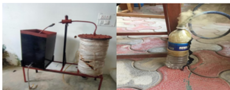
Figure 2. Setup for pyrolysis process of waste plastic into plastic oil (hydrocarbons).
