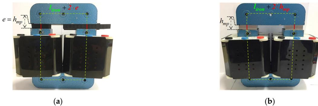
**Figure 18.** Electromagnet’s characterization in terms of power & validation of Ampère’s theorem: (a)  $P_{em}$ —Electromagnet power consumption, (b)  $P_{tot}$ —Total power.
