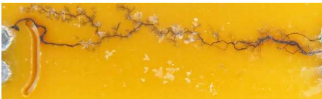
**Figure 20.** Carbonization channel through a PCB with an ionic contamination concentration of  $100 \mu\text{g}/\text{cm}^2$  within 10 min under a 7 kV applied voltage and 85 °C/85% RH.
