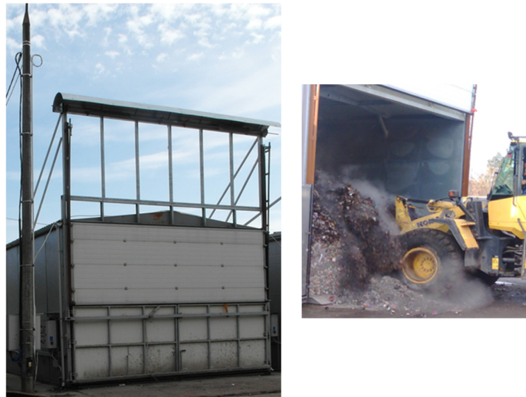
Figure 2. The industrial reactor—the unloading of waste after 14 days of biodrying.
