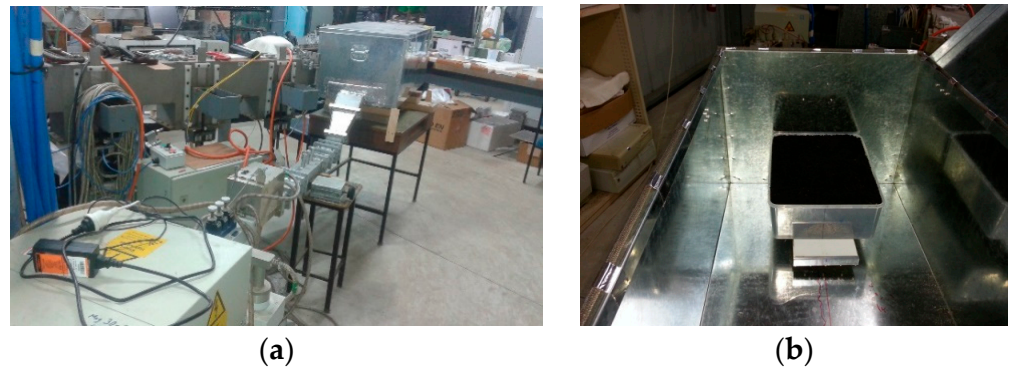
Figure 3. (a) Applicator (inside of metal box) connected to a 30 kW MW generator, operating at 2.45 GHz and (b) showing the soil sample set up on the applicator inside a metal box, which prevented stray radiation of microwave energy.
