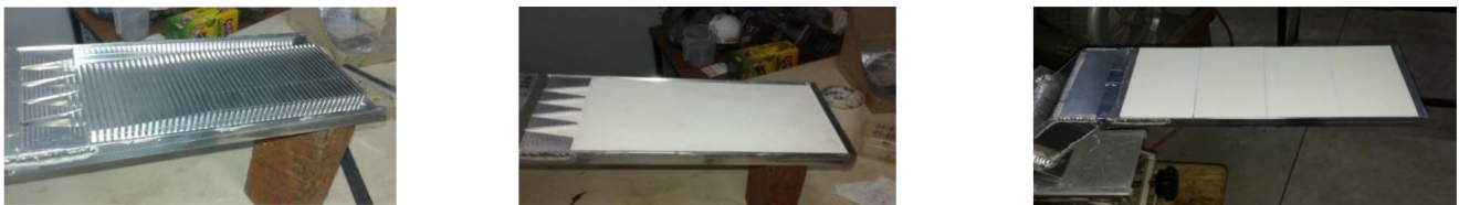
Figure 2. Comb applicator ( left ) and ceramic applicator ( middle ) without ceramic plates, applicator covered with ceramic plates 3 \text{ mm} \times 84 \text{ mm} \times 146 \text{ mm} —4 pieces ( right ).
