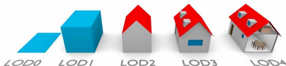
Figure 7. Subsequent levels of detail for building representation in CityGML models [58].
