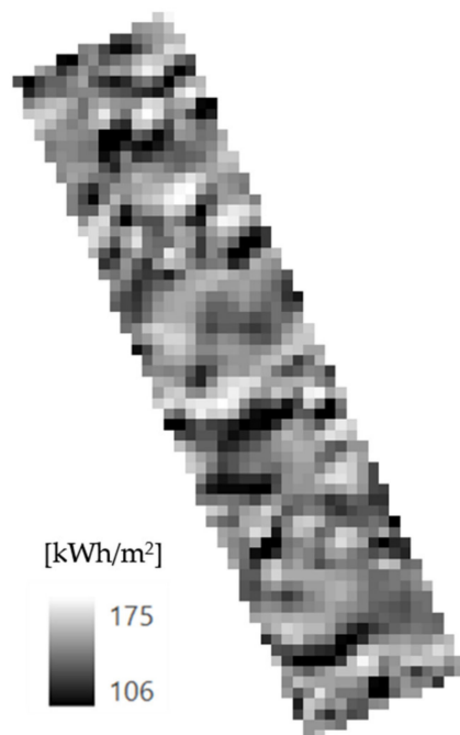
Figure 16. Solar potential values ( \text{kWh}/\text{m}^2 ) obtained for the Rondo ONZ 04 bus shelter, calculated for 10:30 A.M. on 22 June 2020.
