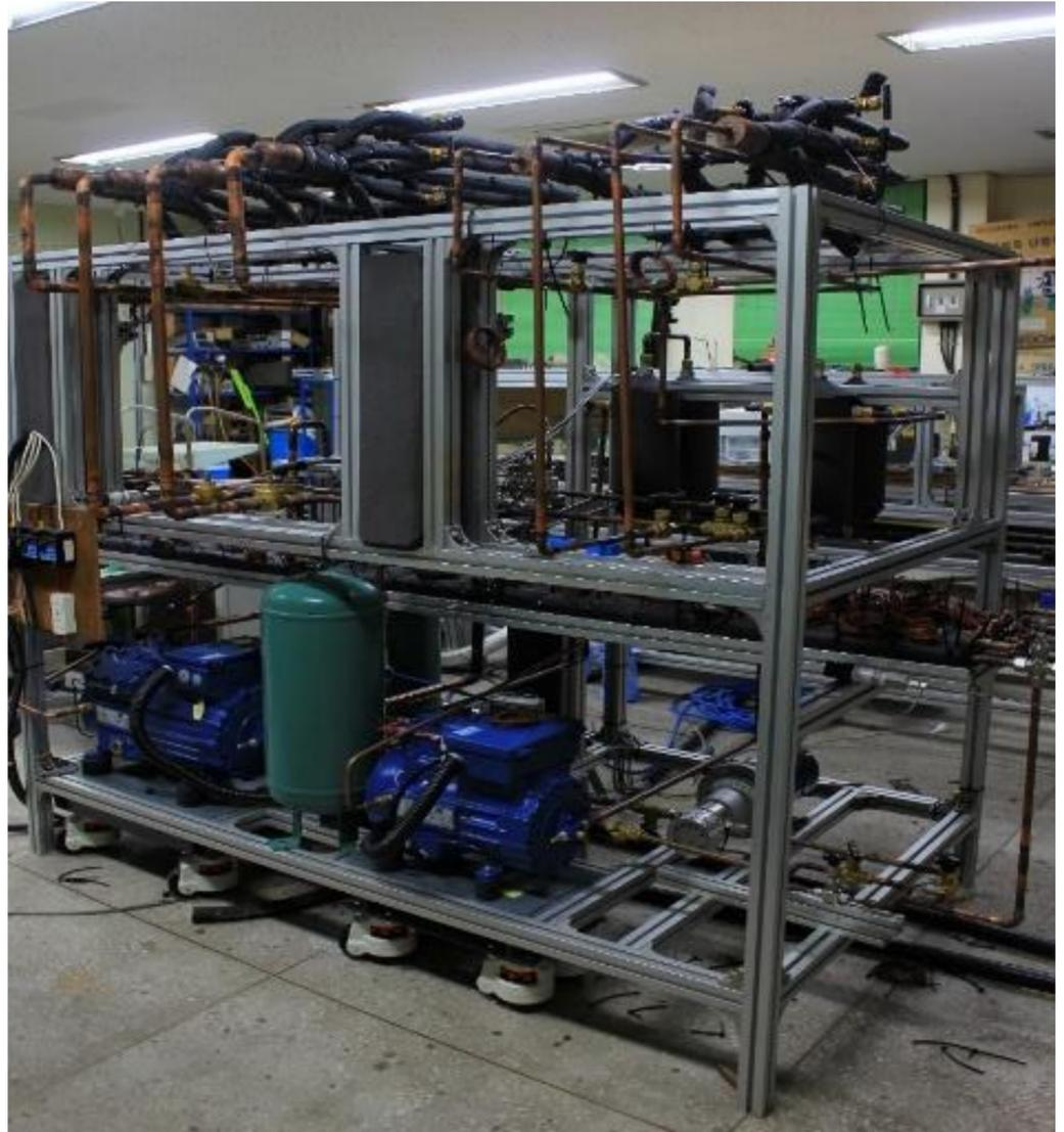
**Figure 1.** Photograph of the experimental apparatus for the CRS using R744.
