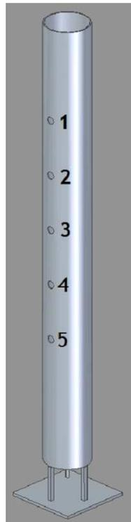
**Figure 3.** Measurement points located on the torch.
