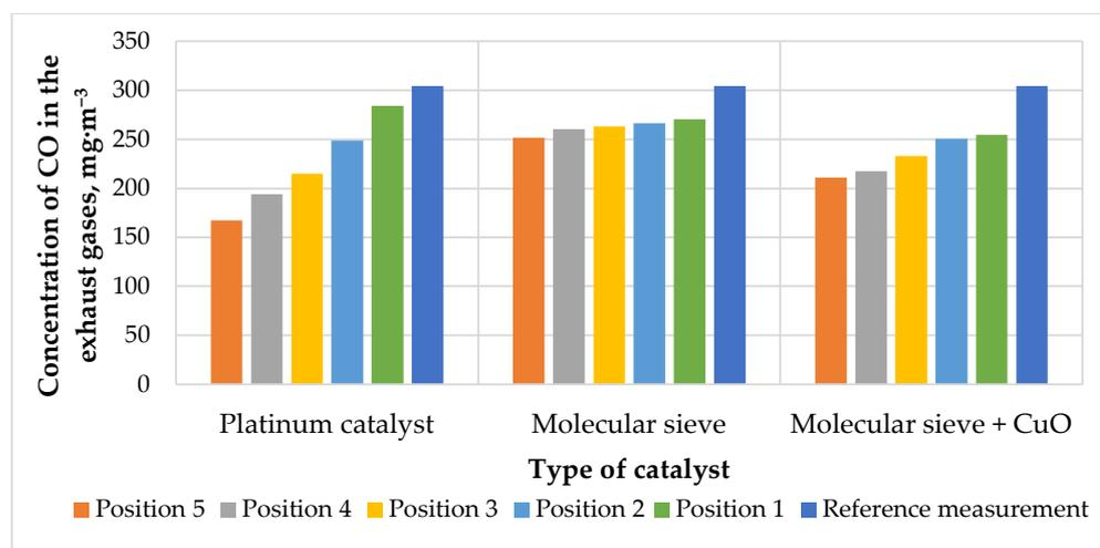
**Figure 6.** CO concentration in exhaust gases depending on the type and location of the catalyst.
