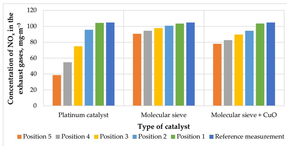
**Figure 7.** NO<sub>x</sub> concentration in exhaust gases depending on the type and location of the catalyst.
