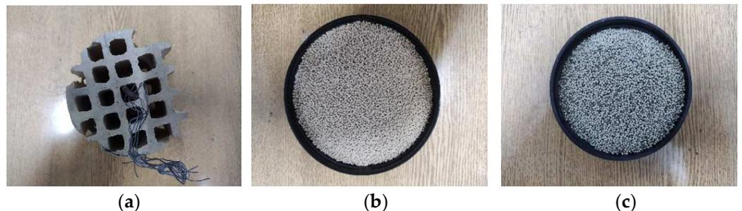
**Figure 4.** Catalysts used in the measurements: (a) platinum catalyst on ceramic carrier; (b) molecular sieve; (c) molecular sieve with copper(II) oxide.
