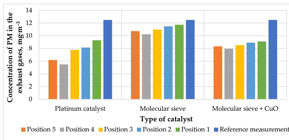
**Figure 8.** PM concentration in exhaust gases depending on the type and location of the catalyst.
