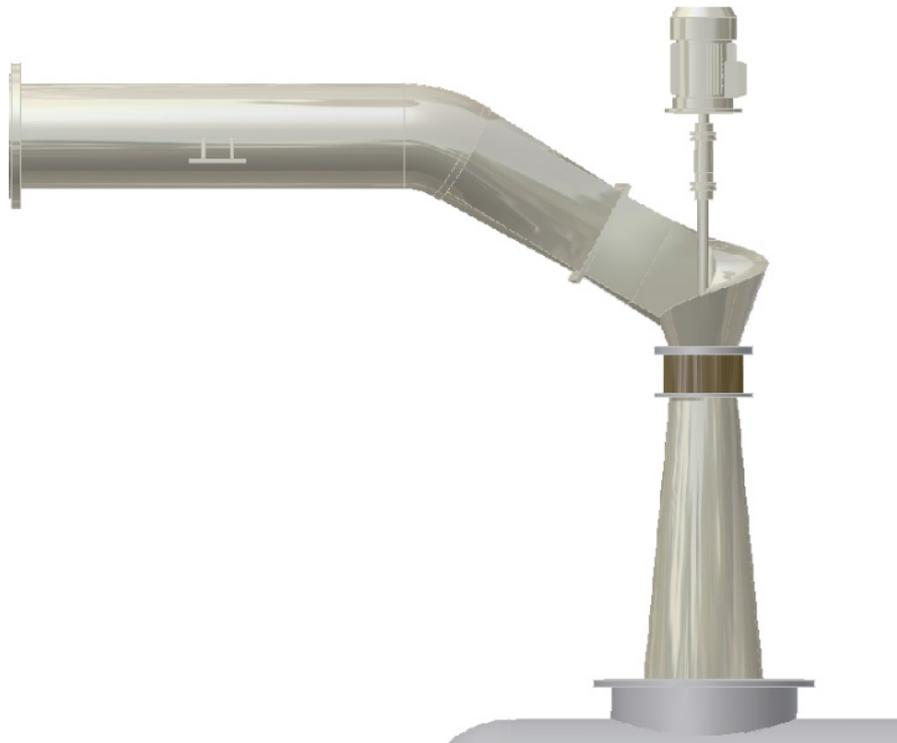
**Figure 5.** Model of a semi-Kaplan hydraulic turbine with a non-classical spiral inflow of water onto the runner.
