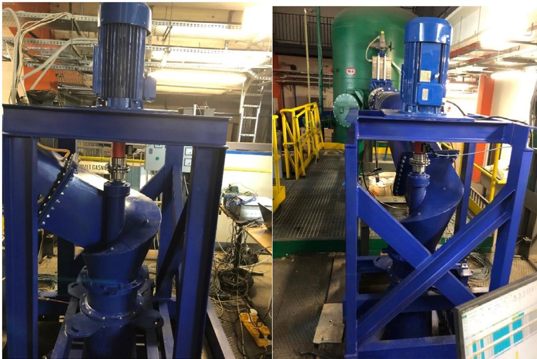
**Figure 11.** Views from the side (left) and from the side opposite to the water inflow (right) of the intake system, supply spiral and runner segment of the model semi-Kaplan turbine.
