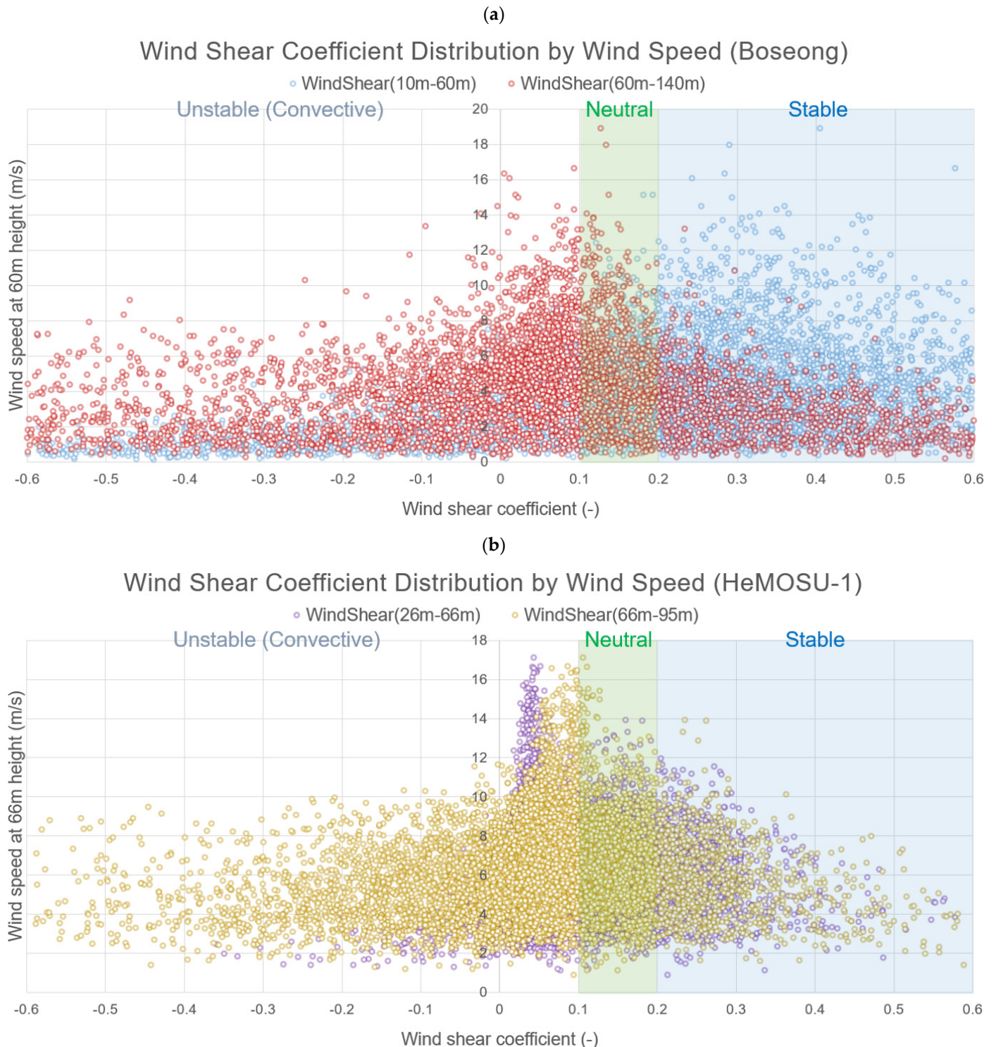
Figure 10. Wind speed is correlated with wind shear coefficient. (a) Boseong mast (blue-colored circles represent wind shear between 10 m and 60 m; red-colored circles represent wind shear between 60 m and 140 m). (b) HeMOSU-1 mast (purple-colored circles represent wind shear between 26 m and 66 m; yellow-colored circles represent wind shear between 66 m and 95 m).
