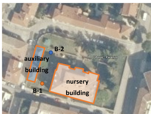
Figure 5. The positions of buildings and wells (B-1 supply well, B-2 return well).
