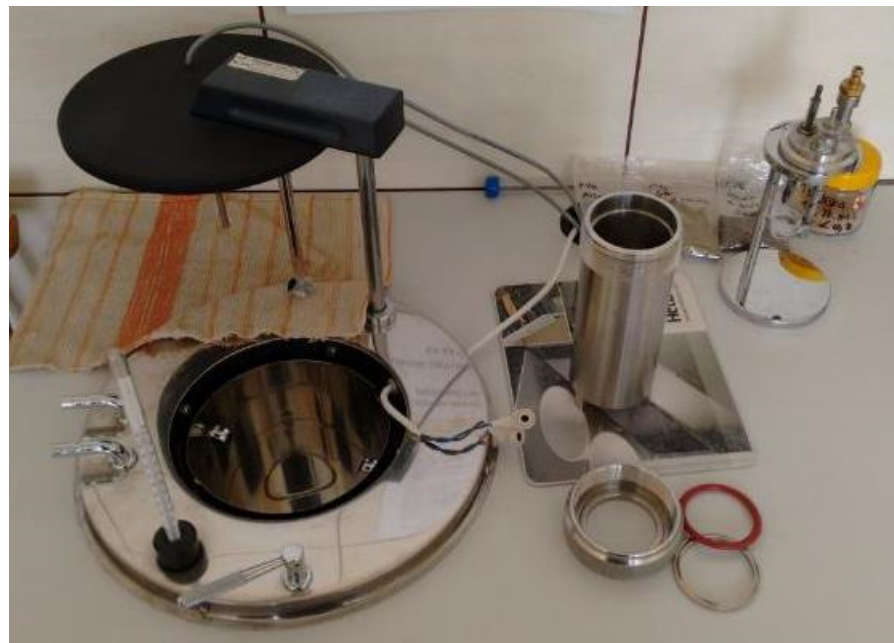
Figure 3. An overall view of the research site for calorimetric measurements ( left ) calorimeter bomb ( right ). [Source: Authors' original photo].
