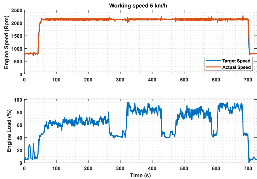
Figure 4. Field test data during work activities with a rotary harrow at 5 km/h.
