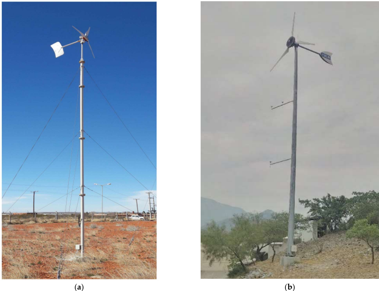
Figure 1. Small wind turbines: 1000 W Eolocal (a) and 5 kW Aeroluz (b).
