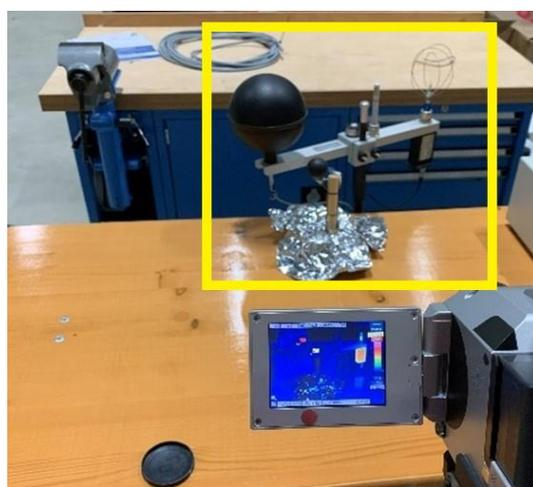
**Figure 2.** Testing configuration with the prototype base covered by aluminium foil.
