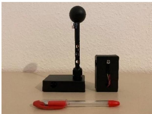
**Figure 1.** Comfort module (on the left side in the above picture); IR module (on the right side in the above picture). A ballpoint pen was placed in the front for scale.
