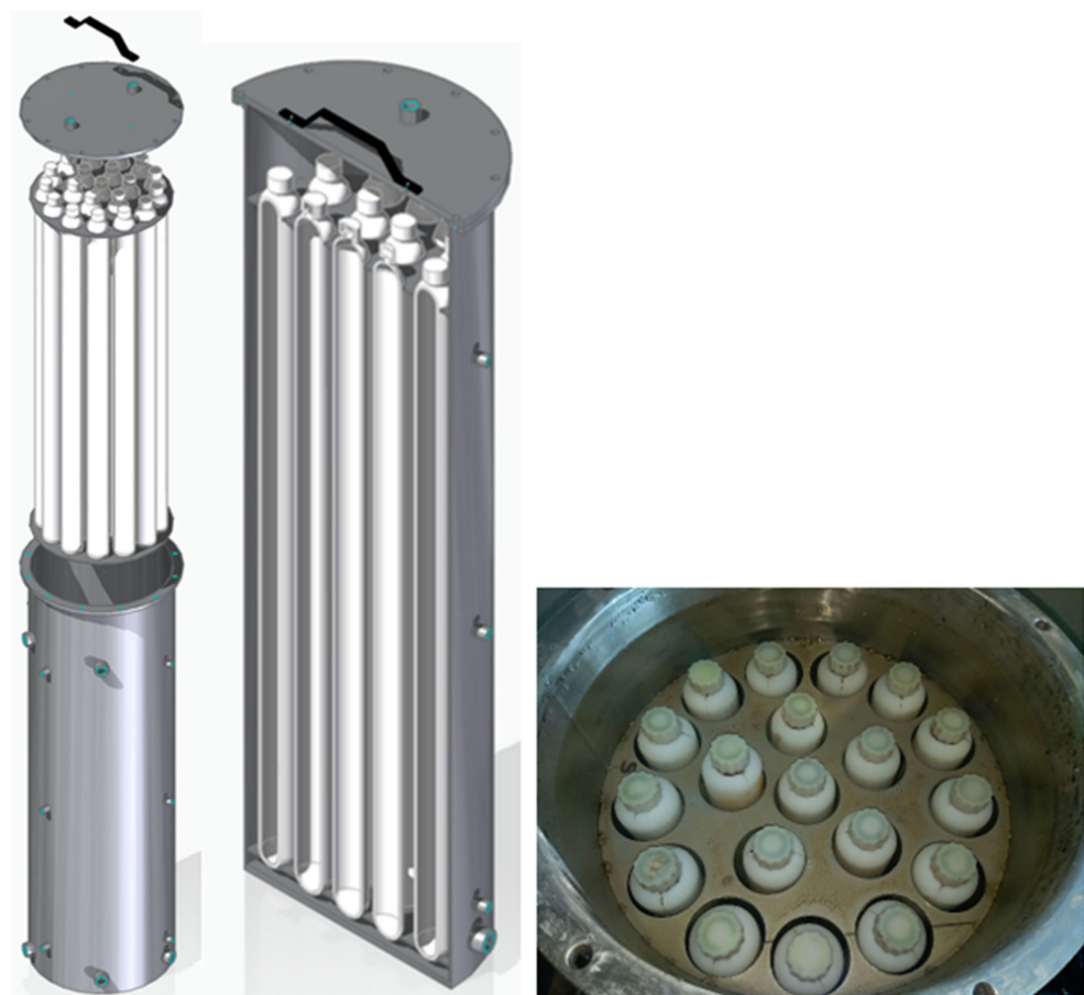
Figure 3. Detailed exploded tri-dimensional view of the designed hybrid sensible/latent storage, left-hand side, section of the internal macro-capsules' arrangement, center, and view of the capsules inserted inside the storage, right-hand side.
