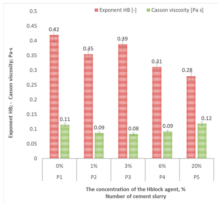
Figure 16. Summary of selected test results for rheological parameters of cement slurries (cement class CEM I 42.5R).
