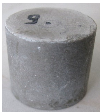
Figure 7. A sample of hardened cement slurry for gas permeability testing.
